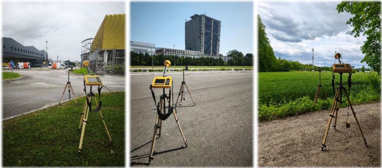
Figure 3.4. The setup for measurements performed in Ljubljana, Slovenia for 5G MaMIMO exposure assessment.
